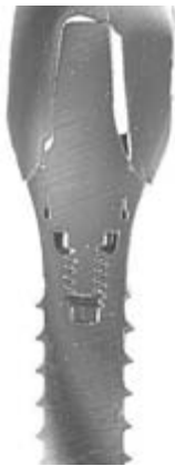
Figure 16.9. A single-stage or transmucosal-type dental implant in cross-section. This is a specimen prepared for laboratory testing and was not used clinically. Note that the crown rests on the external shoulder of the implant body. Load transfer from the occlusal table to the implant is focused on this external shoulder, resulting in inward compressive forces rather than externally directed hoop stresses. This implant design may provide superior resistance to fatigue fracture in areas of heavy occlusal load. This design also provides abutment retrievability and may be used for screw-retained or cement-retained reconstructions.
